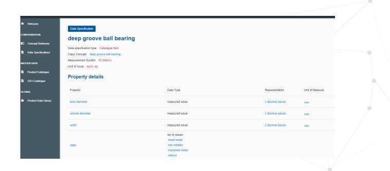
Data Specifications are built from the Concepts - here is the start of a specification for a Deep Groove Ball Bearing
